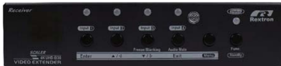
Controls EVBMC-1491L or EVBMV-1391L by Push Buttons ( Wallplate Models as Well )
